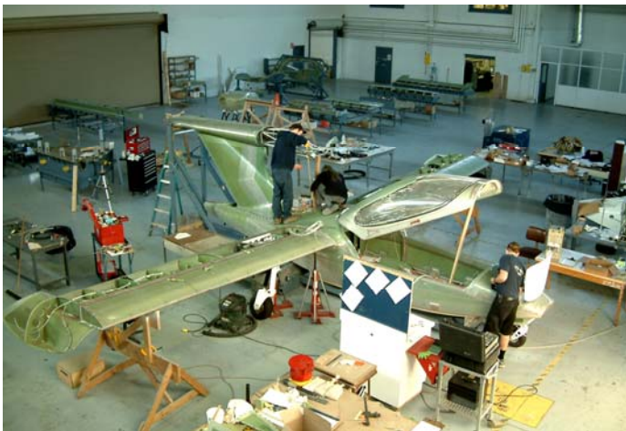
The wings were put back in the assembly fixture to bond the aft top skin.
