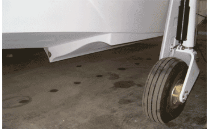
The landing gear is trailing link type. The keel “V” and spray rails are sacrificial.
