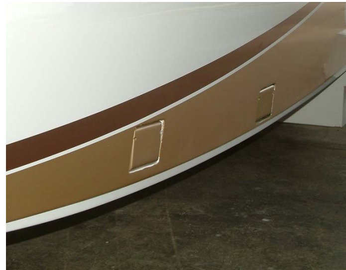
The Seawind has three recessed footstep pockets with spring-loaded covers, one on each side forward and one on the left side aft.
