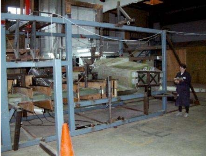
The two wings and the center of the fuselage are upside down for this testing..
