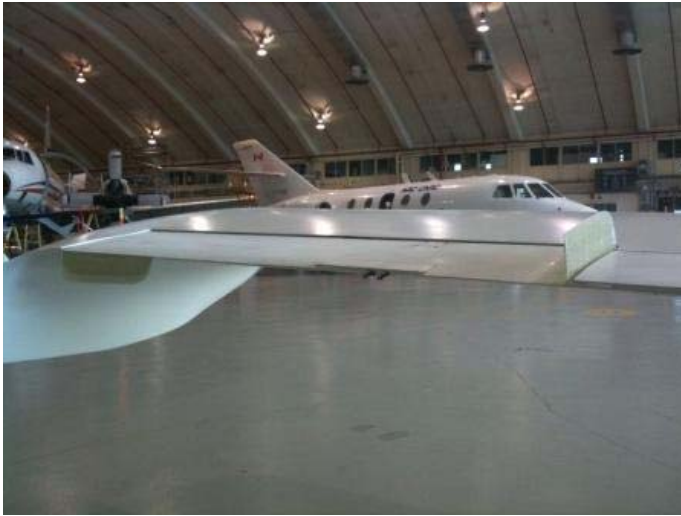
The left wing aileron was modified at the junction with the flap and sponson (wingtip float).
