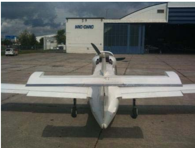
The trailing edge of the elevator and rudder were uniformly modified, including the trim tab.
