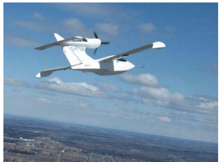
The Seawind departing Ottawa Airport for the final dive speed flutter flight.
